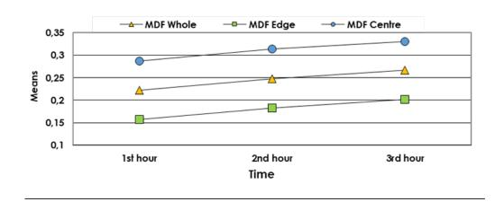
Figure 4. Impact of the different board positions on measurements (MDF)
